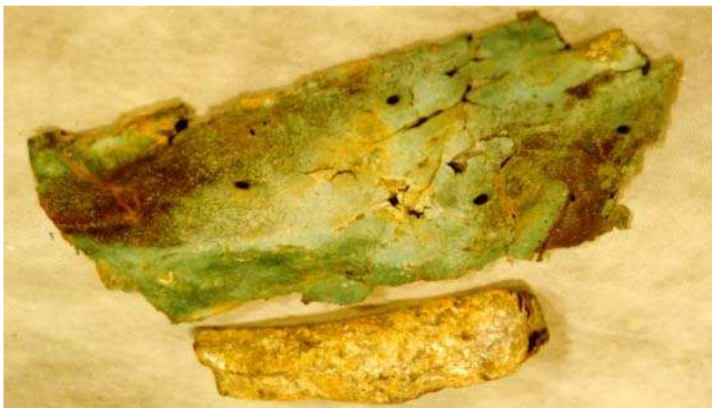
Copper sheathing and lead recovered from the wreck of the St Paul
